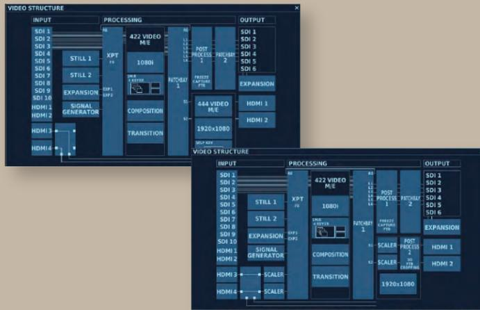
At this screen, you can make video-related settings such as selecting the M/E mode for the 4:2:2 process or changing the connection destinations for HDMI IN 3 and 4. If you want to output HDMI signals with crystal image on large-sized LED and projector displays, you can specify the 4:4:4 process as the connection destination for HDMI IN 3 and 4 here.
