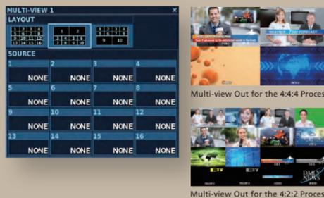
Multi-view is indispensable for single-point monitoring of multiple video feeds. The V-1200HD provides two multi-view outputs, MULTI-VIEW 1 for the 4:2:2 process and MULTI-VIEW 2 for the 4:4:4 process. You can assign video sources for the multi-view screen. Three layout patterns are available for the 4:2:2 process.
