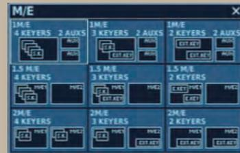
Three M/E modes, 1 M/E, 1.5 M/E and 2 M/E, for the 4:2:2 process are provided to meet the needs of your video production. Each M/E mode has multiple patterns of composition and AUX combinations. Usable composition effects include Self Key (Luminance Key and Chroma Key), External Key and PinP. In cases when you need extra AUXes, you can make settings at the PATCHBAY 1 screen to use unassigned composition buses as AUXes.
