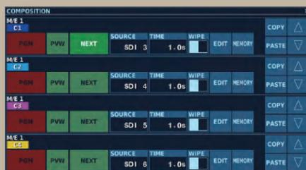
Features for changing priority and for copying and pasting settings are built into the four channels of composition (keyers). You can instantly access preset settings through store and recall operations using four memory banks. The number of keyers available in each M/E differs according to the format selected as the 4:2:2 process format.
